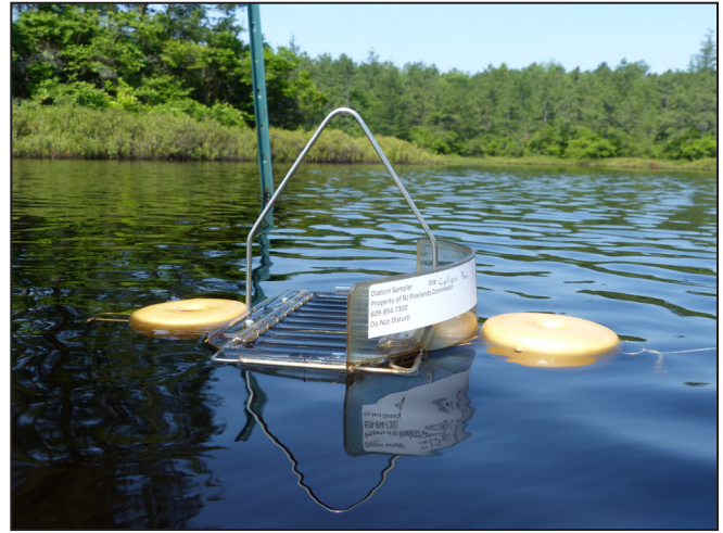
This floating sampler allows diatoms (single-celled algae) in pond water to colonize glass slides during a two-week sample-collection period. Photo/Kim Laidig
